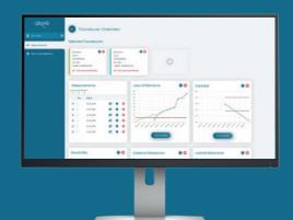
All stored measurements can be found in iQMonitor. The measured transducers are presented in one overview. You can view the measurement values of each transducer in a trend analysis, as well as compare multiple transducers to each other. This way you can track the penetration depth or contrast of your transducer over time. iQMonitor supports user-defined tolerance values. When these are configured, traffic lights will indicate whether your transducer is in, or out of tolerance.
